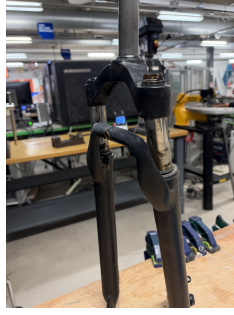
Figure 2: Same front suspension fork after the accident, removed from the bike, with one upper tube clearly bent near the crown while the other side remains straight.”
