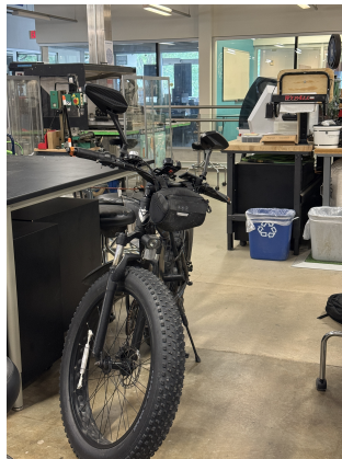
Figure 1: Front suspension fork mounted on the bike before the accident, showing both upper tubes and lower legs straight and aligned.
